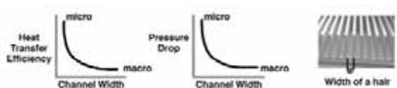
Figure 2b.: Charts show dependence of thermal performance and pressure drop on channel width.
