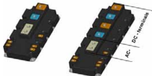
Figure 1: Mechanical outline PrimePACK™2 on the left and PrimePACK™3 on the right side. Both types form a half bridge configuration with 3 connections: DC+, DC- and AC output.
