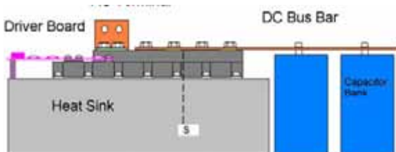
Figure 9: PrimePACK™ linked to a 2 layer busbar. The AC load terminal is screwed to a separate load connector.
