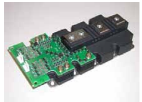
Figure 2: PrimePACK™2 with active booster stage mounted.
